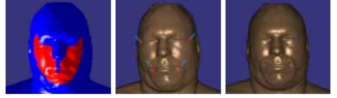
Figure 14: a) Boundary conditions represented as a texture map onto the range data (blue: rigid nodes, red: non-rigid nodes). b) Interactive definition of nodal forces. c) Deformation of the facial shape in accordance with the boundary conditions on the left.
